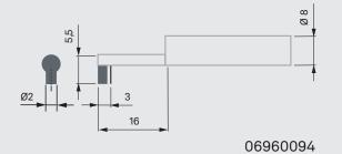
**SB121 probe** For groove of depth < 20 mm
