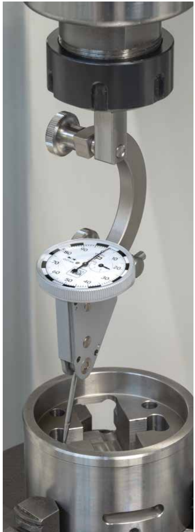
The centering holder allows a large range of movement of the lever-type dial test indicator, useful for measuring at different distances as well as for centering a workpiece on a machine tool.
